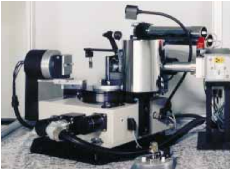
Typical setup of STOE's transmission diffractometer STADI P with linear PSD, transmission sample holder including the sample changer and the curved Ge(111) monochromator beneath its cover.
