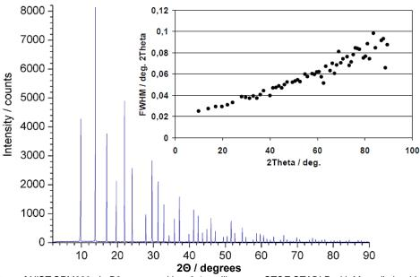
Powder pattern of NIST SRM660a LaB6, measured in a 0.1 capillary on a STOE STADI P with Mo radiation (data point interval 0.01°). Note the low background and the extraordinary FWHMs (for the latter see inlay above, shown as function of 2e).
