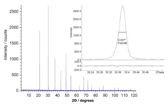
Powder pattern of NIST SRM660a LaB6, measured on a STOE STADI MP with Cu radiation in transmission mode (data point interval 0.009°). Note the good fit and the high resolution shown by the (110) reflection (see inlay above).
