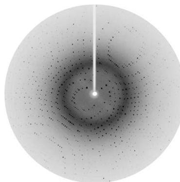
**Fig.2:** Diffraction frame recorded on an elastase crystal. Scan width 1° (Omega), exposure time 300 sec. Crystal-Detector distance 150mm. Resolution at edge (170mm from center): 1.89 Å
