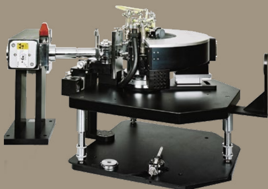
Basic version mounted on a fixed stage with STOE's large IP-PSD, video CCD and tube housing.
