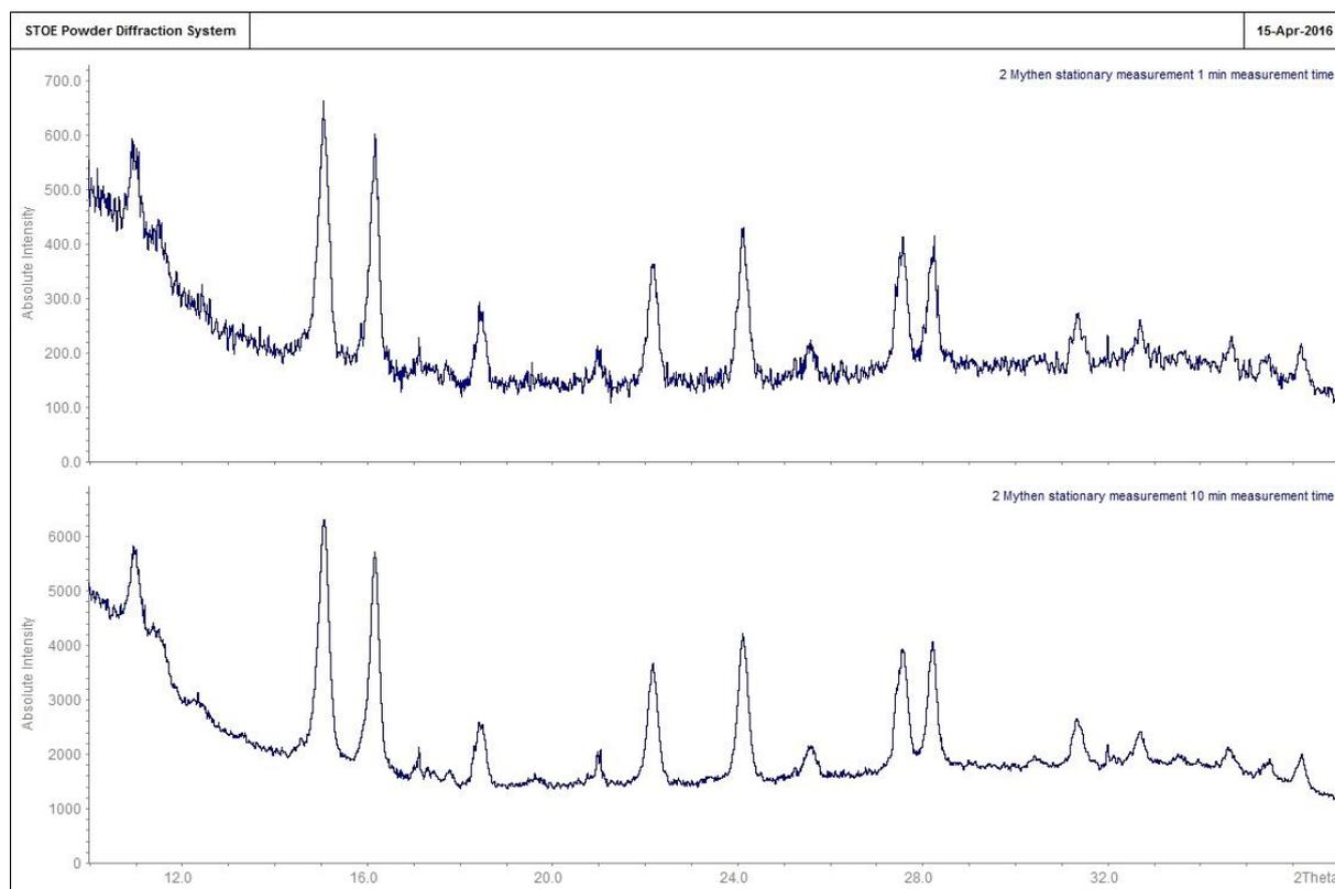
**Figure 3: Measurements simulating a MYTHEN1K dual detector array in stationary measurement mode with ~1 min measurement time (top) and ~10 min measurement time (bottom)**
