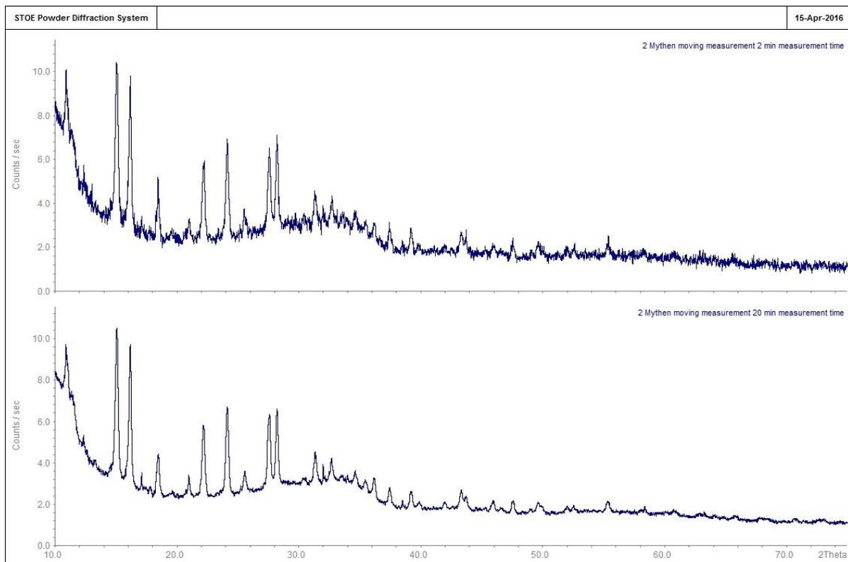
**Figure 4: Measurements simulating 2 MYTHEN1K detectors in a two-step measurement mode; 2 min measurement time (1 min exposure time each step) top and 20 min (10 min exposure time each step) bottom**
