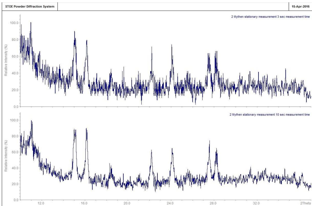
**Figure 2: Measurements simulating a MYTHEN1K dual detector array in stationary measurement mode with 3 sec measurement time (top) and 10 sec measurement time (bottom)**
