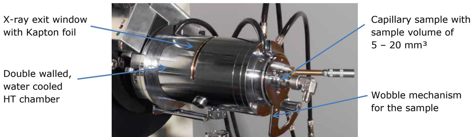
**Figure 1: STOE INSITU HT2 high temperature reaction chamber installed on a vertical STOE STADI P transmission diffractometer using focused pure Molybdenum  $K_{\alpha 1}$  radiation.**
