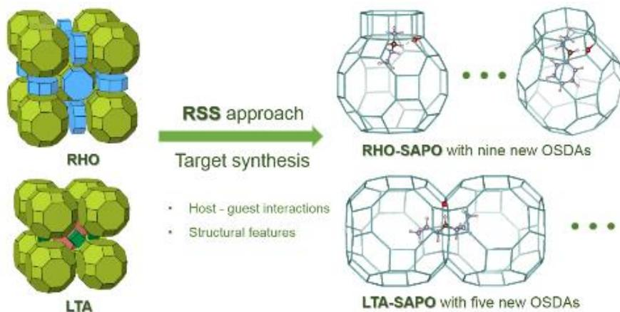
Figure 1. Targeted synthesis of DNL-6 and SAPO-42 by utilizing the RSS method.
