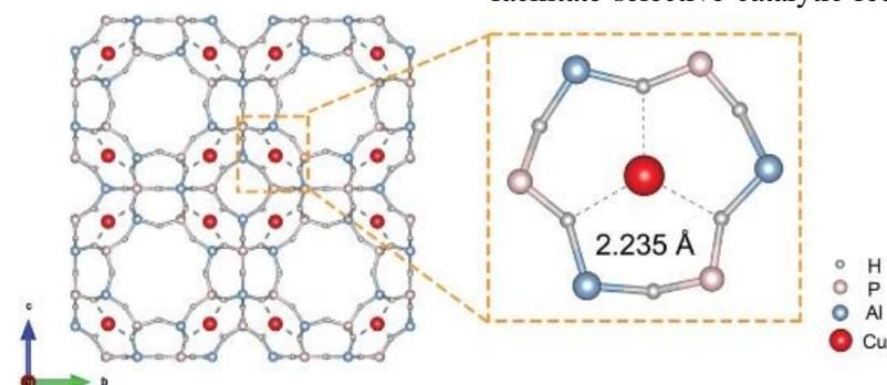
Figure 3. The locations of active Cu<sup>2+</sup> ions in Cu-SAPO-42 catalyst.
