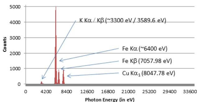
Figure 1: Photon energy spectrum of  $\text{K}_3[\text{Fe}(\text{CN})_6]$  after 15 h exposure time measured with a Si PIN diode point detector and 8.0 keV excitation energy (Cu  $\text{K}\alpha_1$ ); clear separation of  $\text{K}\alpha$  and  $\text{K}\beta$  of Fe is visible.
