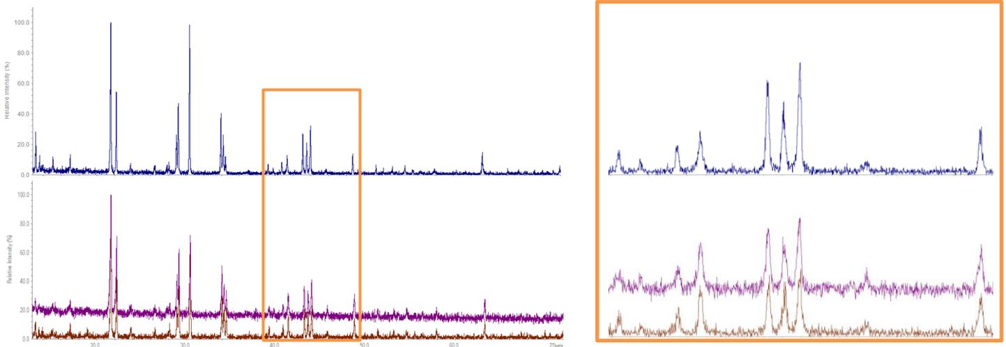
Figure 3: Measurements of  $\text{K}_3[\text{Fe}(\text{CN})_6]$  with  $\text{Cu } K\alpha_1$  radiation; Si PIN diode point detector (blue) in comparison to scintillation counter with (brown) and without (purple) secondary beam monochromator after 17h measurement time. A close-up between  $41$  and  $49^\circ 2\theta$  shows an improved signal-to-noise ratio for the Si PIN diode point detector compared to the scintillation counter.
