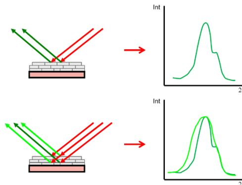
*Comparison between a strong (top) and weak absorbing material (bottom) in reflection geometry.*
