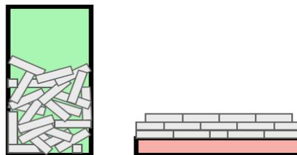
*Plane crystallites in a capillary (left) and the same particles pressed in a reflection sample holder (right).*
