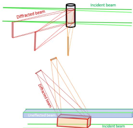
*Comparison of beam path in transmission (above) and reflection geometry (below).*
